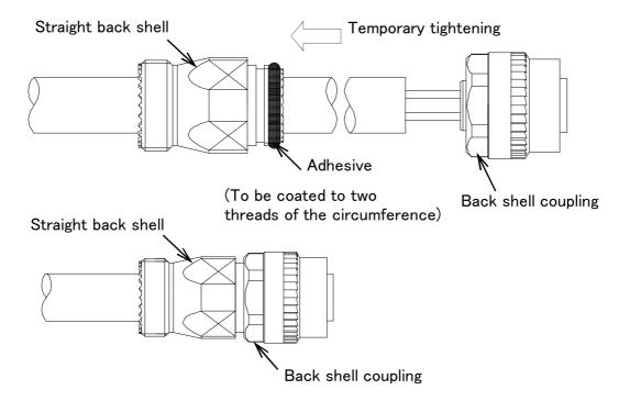
\* When tightening temporarily, match the concavity and convexity of the plug shell with those shell.of the straigh back shell.
