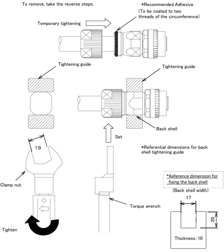
● Jig/Tool Used: Clamp nut wrench (357J-51334T)
