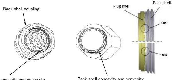
Plug shell concavity and convexity
