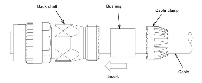
Note! After the Bushing insert, confirm that cable position should be inside of Bushing.
