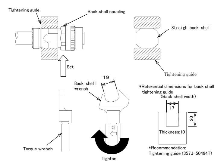
Note! To change the straigh back shell, do it by changing the engaging position of the concavity and convexity of the plug shell and the back shell.
