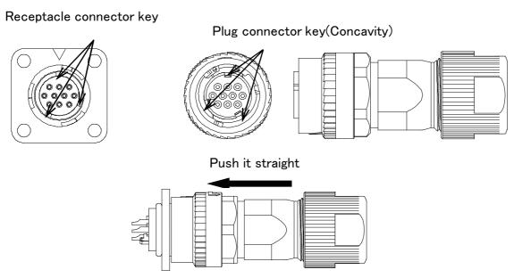
\*To remove, rotate the coupling and pull out to straight.
