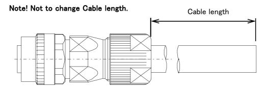
\*Cable length after cutting =35 $\pm$ 0.5mm for CM10-SPXXS(D6) + cable length =35 $\pm$ 0.5mm + cable length
